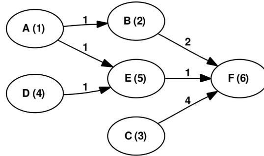
**Figure 1. Example of a static task graph. Values in parenthesis inside the nodes represent execution time, and values at edges represent communication sizes. The communication time will be determined by the interconnect, its availability and data size.**
